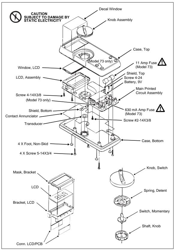
Figure 1. 70/73 Assembly Details
