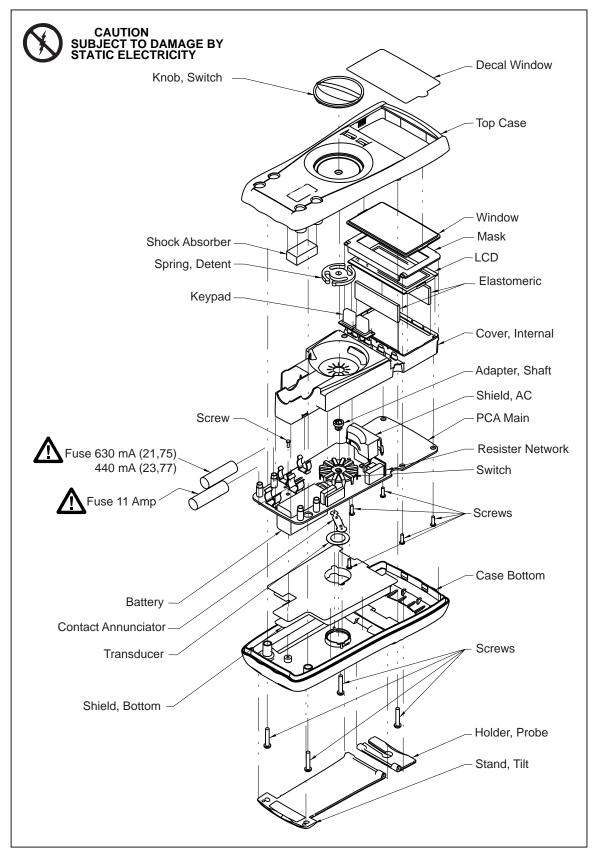
Figure 2. 77/75/23/21 Assembly Details
